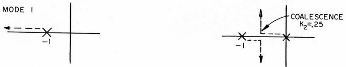
Fig. 25 - Mode 1 and Mode 2 Pole-Zero Plots for One Pole
