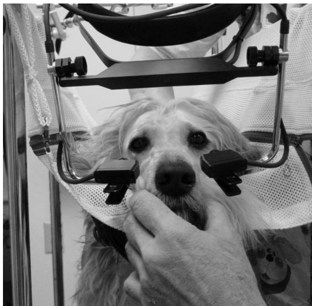
FIGURE 1. EyeLink II (SR Research Ltd., Mississauga, Ontario, Canada) camera setup. The dog's head is supported from below and stabilized from behind.
