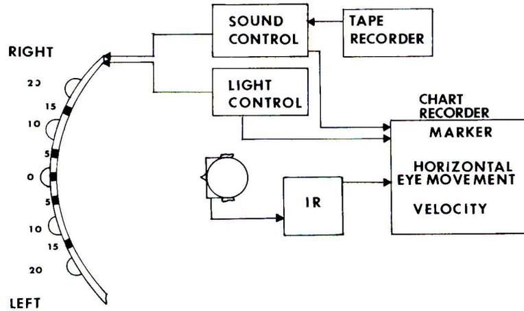
FIG. 1. Block diagram of the experimental apparatus.
