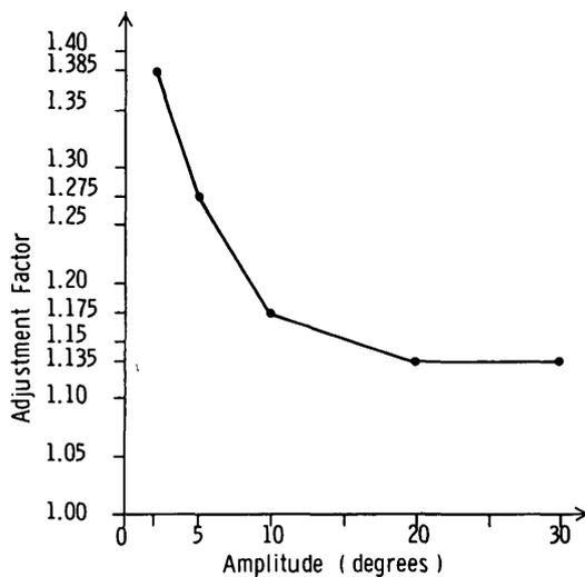
**Fig. 1.** Adjustment curve indicating the relationship between infrared reflection and conventional EOG techniques. More accurate saccadic peak velocities may be obtained from those measured using 25 Hz. bandwidth EOG by multiplying the latter by the adjustment factor indicated for each saccadic amplitude.
