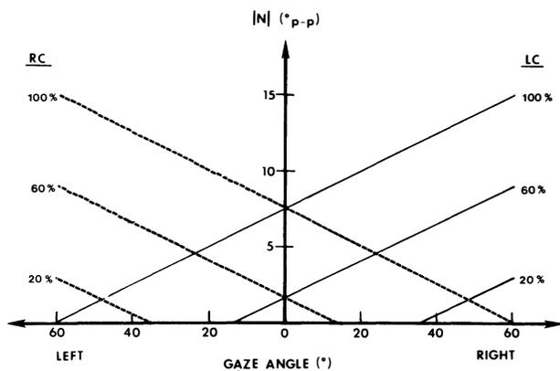
Fig. 5. Plots of variations of nystagmus amplitude as a function of gaze angle and the amount of simulated semicircular canal dysfunction. LC - Left canal; RC - Right canal.<sup>2</sup>
