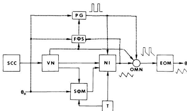
Fig. 3. Functional block diagram of the model. Solid lines represent slow phase generation; dashed lines represent fast phase aspects. SCC - Semicircular canal; VN - Vestibular nuclei; NI - Neural integrator; OMN - Ocular motor nuclei; EOM - Extraocular muscles;  $\Theta_D$  - Desired gaze angle;  $\Theta_E$  - Eye (gaze) angle; PG - Pulse generator; F $\Phi$ S - Fast phase stimulator; S $\Phi$ M - Slow phase modulator; T - Central tonic input.<sup>2</sup>
